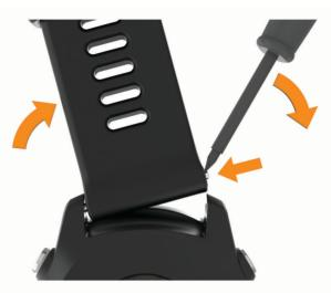
**NOTE:** Make sure the band is secure. The watch pin should align with the holes on the device.
